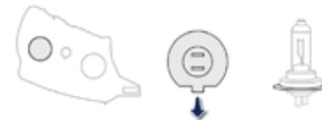
To reassemble, carry out these operations in reverse order, positioning the alignment lug at the bottom.
