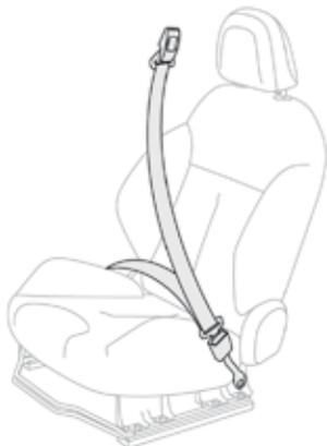
The front seat belts are fitted with a pretensioning and force limiting system. This system improves safety in the front seats in the event of a front or side impact. Depending on the severity of the impact, the pretensioning system instantly tightens the seat belts against the body of the occupants. The pretensioning seat belts are active when the ignition is on. The force limiter reduces the pressure of the seat belt on the chest of the occupant, so improving their protection.
