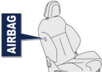
System which protects the driver and front passenger in the event of a serious side impact in order to limit the risk of injury to the chest, between the hip and the shoulder. Each lateral airbag is fitted in the seat backrest frame, door side.
