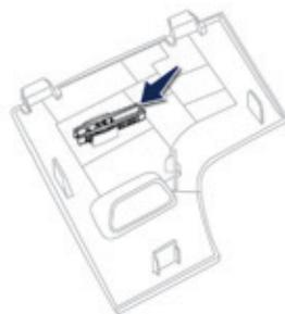
The extraction tweezers is fitted to the back of the fusebox cover located inside the glove box.
