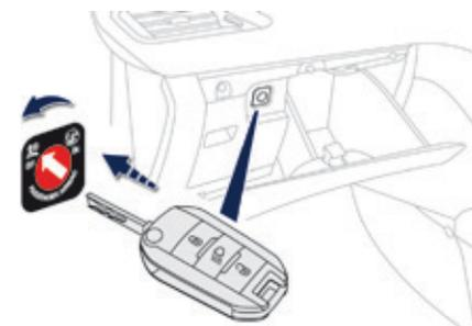
Only the passenger's front airbag can be deactivated.
