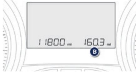
System that measures the distance travelled (daily, for example) since it was last reset by the driver. The trip recorder is displayed in zone **B** of the instrument panel screen.
