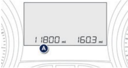
System that measures the total distance travelled by the vehicle during its life. The total distance is displayed in zone **A** of the instrument panel screen.
