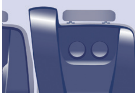
The seat backs of the centre seats are designed with cup holder and storage recesses.
